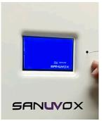
3. First turn ON the power switch and then, press the reset button. You have 5 seconds from the moment the unit is powered to press the reset button to activate the airflow detection. Every time you press the button you will notice the word "AIR" appears or disappears from the bottom right corner of the LCD screen. Once "AIR" appears on the screen, wait for the lamp to turn on so that the setting is saved.
