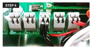
6. After the test is completed, unplug the unit and replace the wires in their original position. Black wire from the power cord connects into L and white wire from the cord connects into N. Black wire going to the ballast connects into B-L and white wire going to the ballast connects into B-N.
