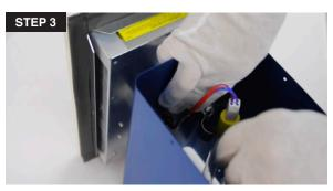
3. Remove the old UV lamp from the lamp socket by opening the retaining clamp and pulling the UV lamp out of the reflector chamber.
