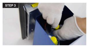
3. While holding the porcelain end-cap (with 4 pins) in the clamp, carefully push the white connector onto the four pins. The plug is designed so that it can only be installed one way. You may have to rotate the socket 90° to line up the pins with the holes. The connector will fit into position.
