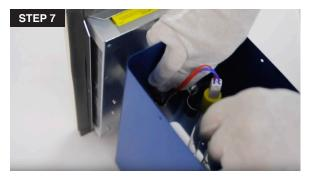
7. Slide the **UV lamp porcelain end-cap (with 4 pins)** in the aluminum tube of the unit, then through the clamp.
