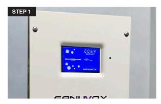
1. To reset the lamp timer the unit needs to be powered and turned ON. The LCD status should be on 'Stand-by' or 'Active'.
