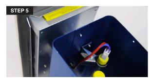
5. Once the UV lamp is inserted, release the clamp to fix the lamp in place.
