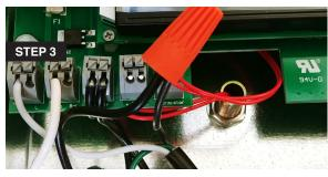
3. Disconnect L and B-L and join them together using twist-on wire connectors
