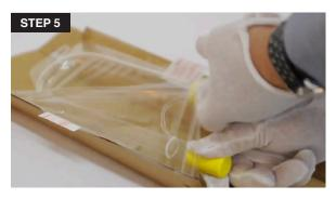
Carefully slide the new UV lamp out from the cardboard sleeve. Be sure
