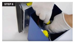
6. While holding the porcelain end-cap (with 4 pins) in the clamp, carefully push the white connector onto the four pins. The plug is designed so that it can only be installed one way. You may have to rotate the socket 90° to line up the pins with the holes. The connector will fit into position.
