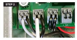
2. Locate the power input to the circuit board (N,L) as well as the ballast input (B-N,B-L).
