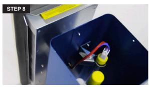
8. Once the UV lamp is inserted, release the clamp to fix the lamp in place.
