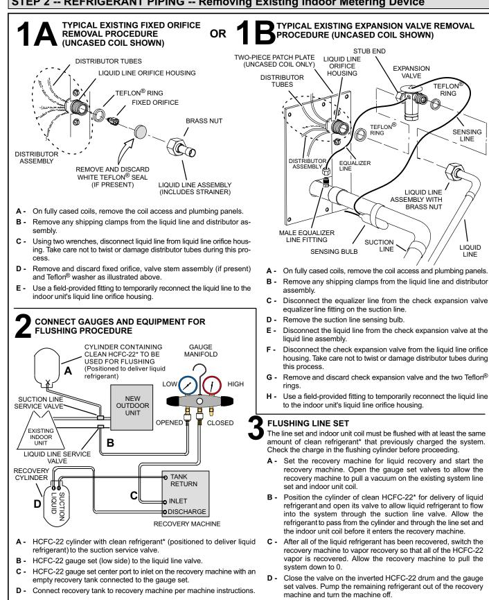
\*IMPORTANT - Clean refrigerant is any refrigerant in a system that has not had compressor burn out. If the system has experienced burn out, it is recommended that the existing line set and indoor coil be replaced.
