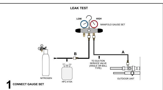
A - Connect the high pressure hose of an HFC-410A manifold gauge set to the suction valve service port.
