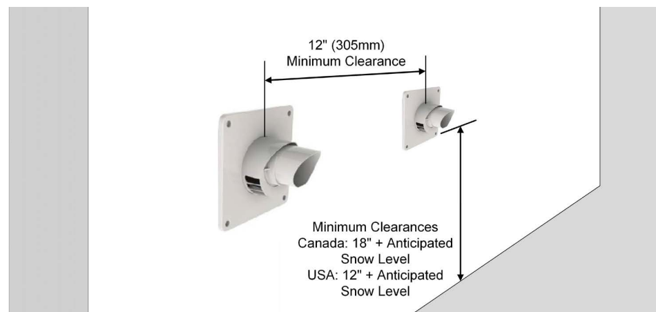
Figure 11a: Horizontal Concentric Termination - Two Kits
